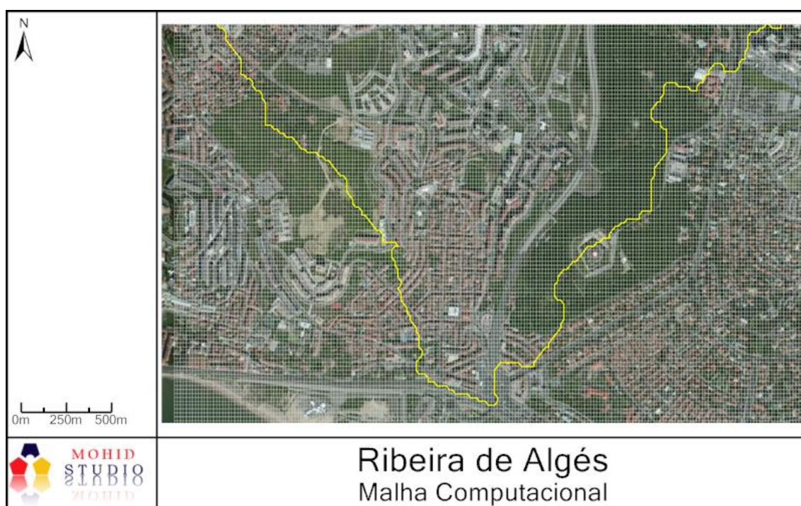
Figure 8: Zoom of the computational grid used for MOHID Land near the outlet
