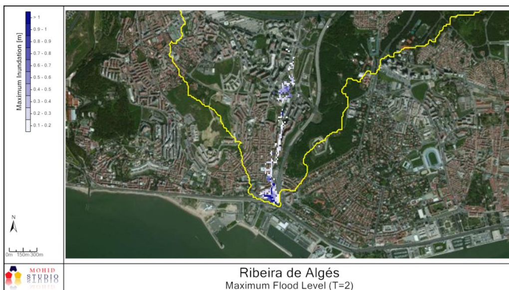
Figure 13: Maximum expected inundation depth (T=2 years)
